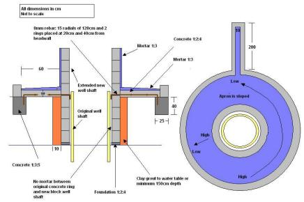
Figure 6: Flood-proofed well, Madagascar - raised headwall built to the exterior of the original well shaft and clay grout Eric Fewster, Medair
