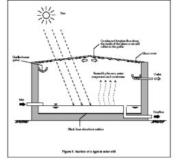
Figure 5: Typical single basin solar still Shaw, R. (ed) (1999). *Running Water: more technical briefs on health, water and sanitation*. Practical Action Publishing, London.
