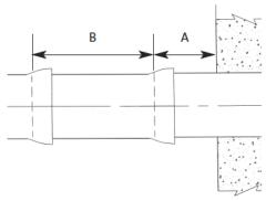
Figure 15: Rocker pipes Saint-Gobain Pipelines (2006) Pipe & Fittings - Water & Sewer: Design Guide. Saint-Gobain, Ilkeston, UK
