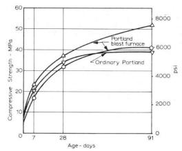
Figure 3: Concrete strength with curing
