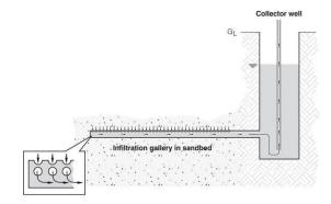
Figure 12: Infiltration gallery Image courtesy of WEDC. © Ken Chatterton. In: Hussey, S.W. (2007) Water from sand rivers: guidelines for abstraction. WEDC, Loughborough University, UK.
