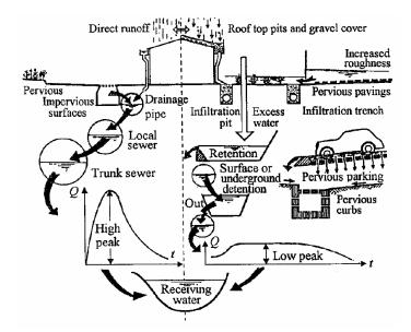
Figure 20: Two concepts for urban drainage – without or with SUDS Maksimovic, C. (1996) Measurements of Water Quantity in Urban Areas. In: WMO. Rain and Floods in our Cities – Gauging the Problem. WMO/TD – No. 741.
