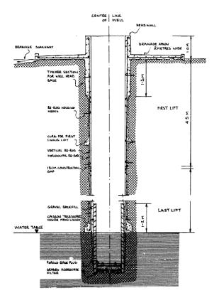
Figure 10: Hand-dug well with telescopic lining Watt, S.B.; Wood, W.E. (1979) Hand Dug Wells and their Construction. IT, London, UK.
