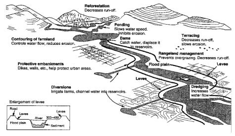
Figure 4: Flood control structures and actions Reed. S.B. (1997) Introduction to hazards. 3<sup>rd</sup> Edition. UNDP. p.90
