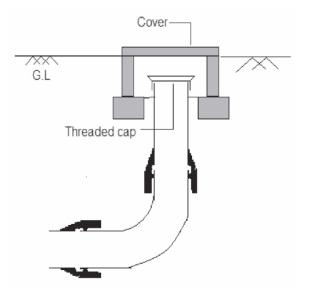
Figure 18: Rodding eye built into the wastewater network Harvey, P. (2007) Excreta Disposal in Emergencies: A Field Manual. WEDC, Loughborough University, UK.
